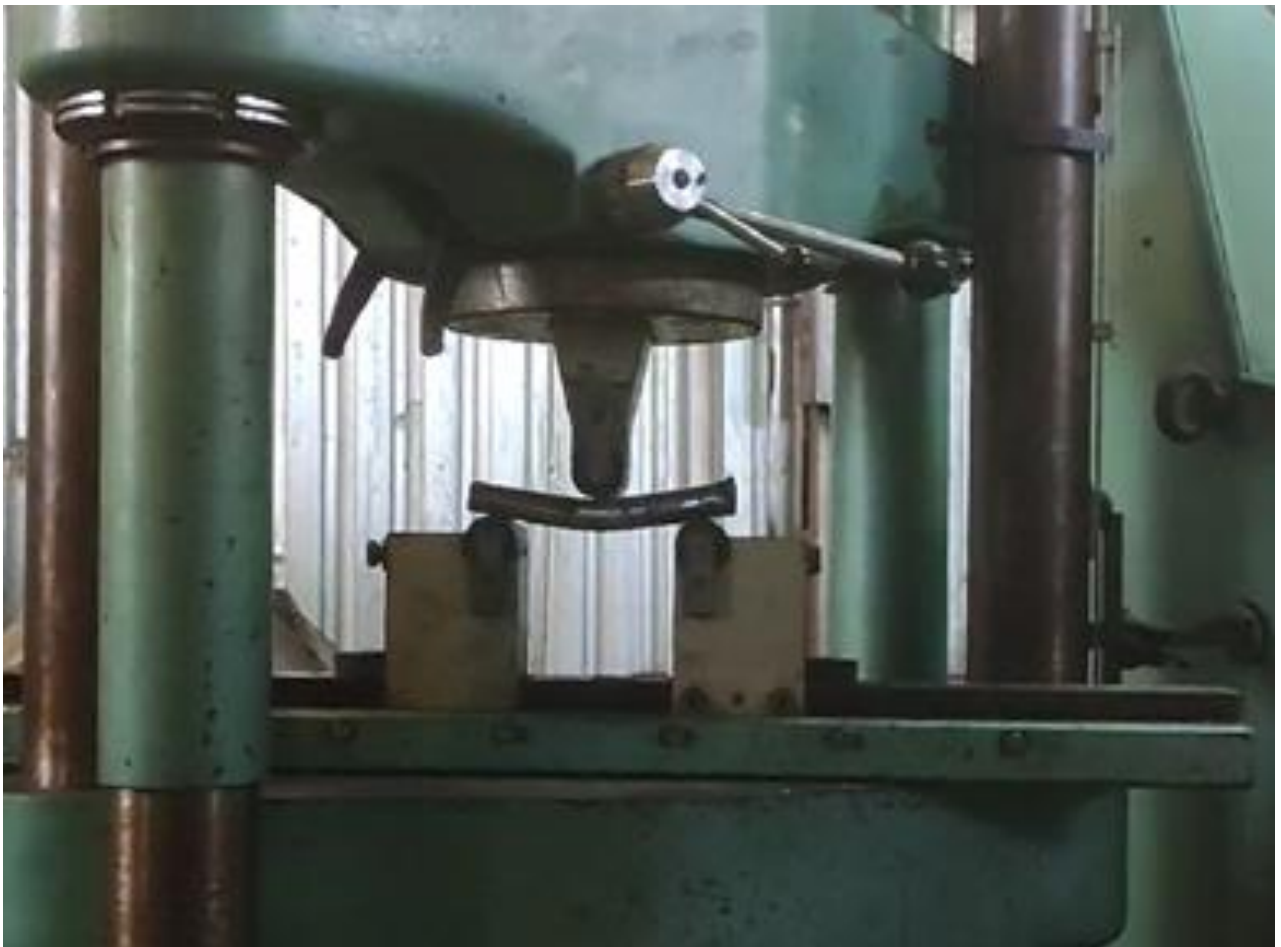
Figure 1 - Ductile cast-iron made with Sarytogan Graphite Micro80C passing bending tests
