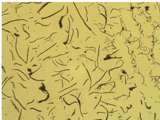
Figure 2 - Photo micrographs of grey cast-iron made with Sarytogan "Micro 80C" Graphite
