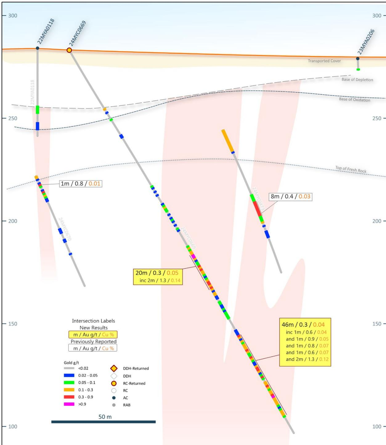
**Figure 9: Fiamá deposit NW-SE cross-section 423,990mE (refer to Figures 1, 2 and 5 for location) showing gold±copper drill intercepts, with the deposit open down dip ± along strike for multiple zones of mineralisation. NB: 50m elevation (RL) grid, looking toward 052° GDA2020 / MGA Zone 51 Grid.**
