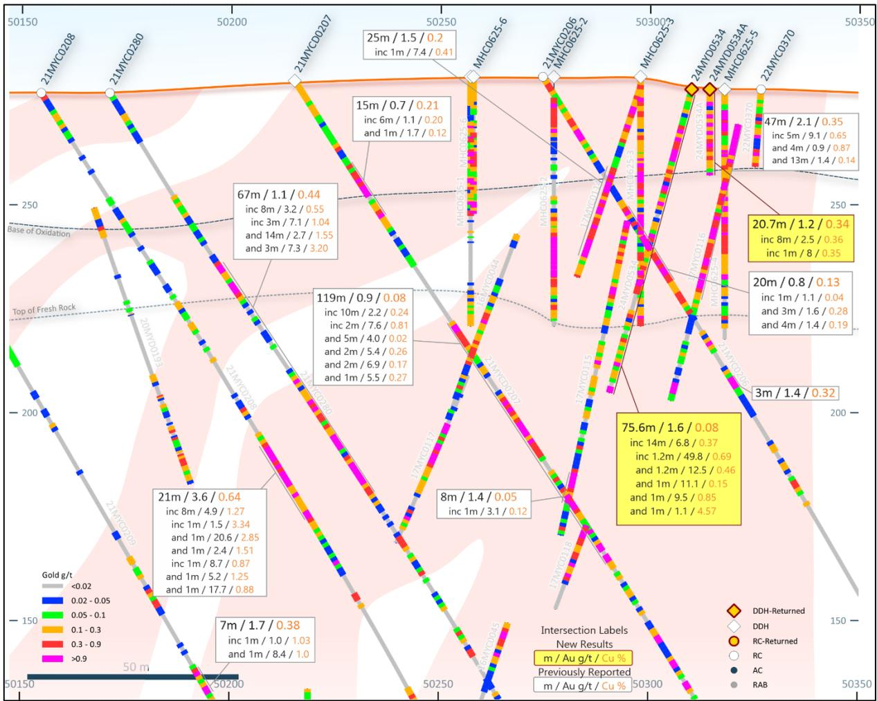
**Figure 4: Minyari deposit 100,625mN east-west cross-section (refer to Figures 1 and 2 for location) showing gold±copper drill intercepts. NB: 50m elevation (RL) and 50m Local Grid northing co-ordinates, looking toward Local Grid 360° (or 328° GDA2020 / MGA Zone 51 Grid).**
