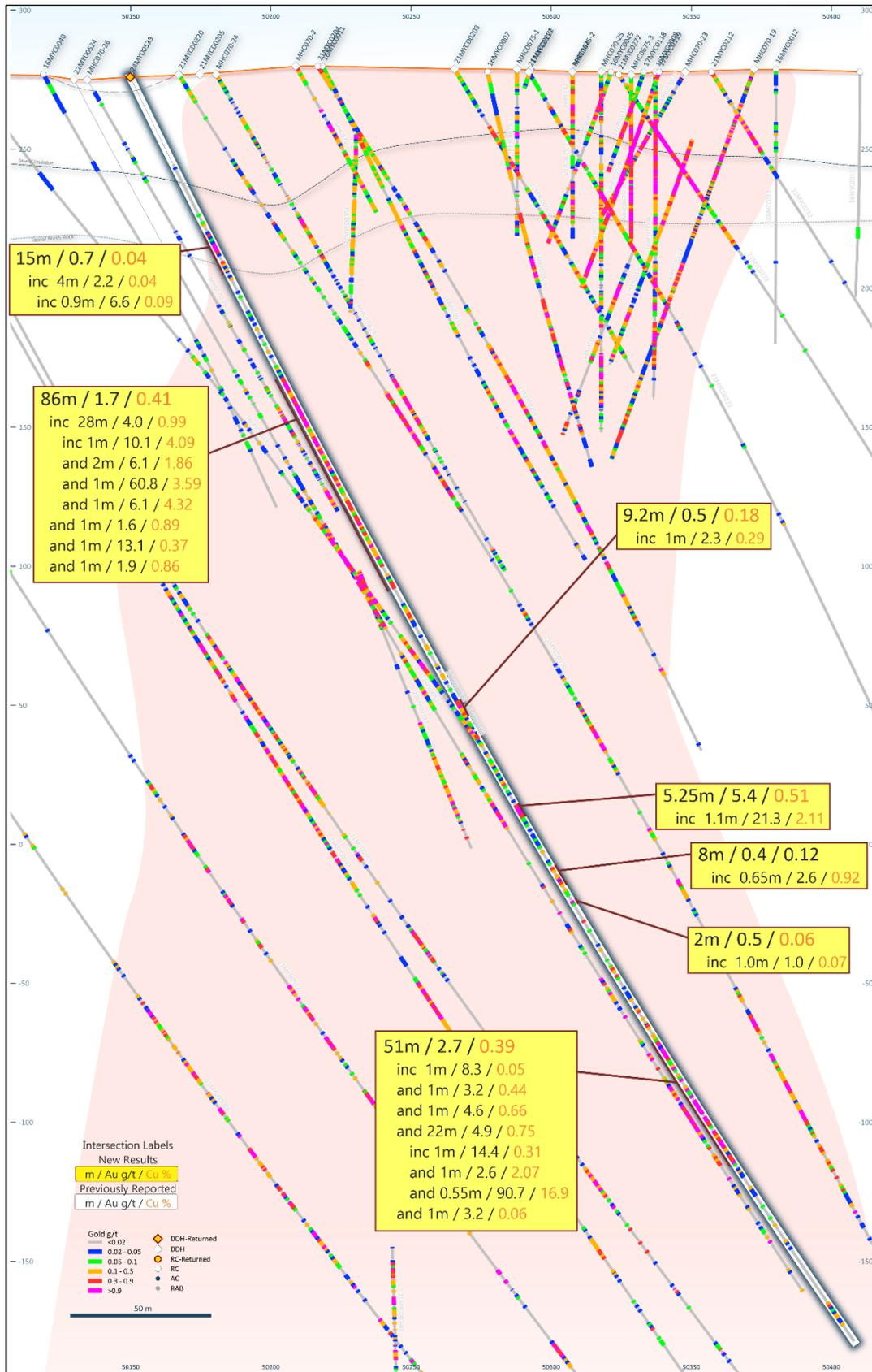
**Figure 3: Minyari deposit 100,700mN east-west cross-section (refer to Figures 1 and 2 for location) showing gold±copper drill intercepts. NB: 50m elevation (RL) and 50m Local Grid northing co-ordinates, looking toward Local Grid 360° (or 328° GDA2020 / MGA Zone 51 Grid).**
