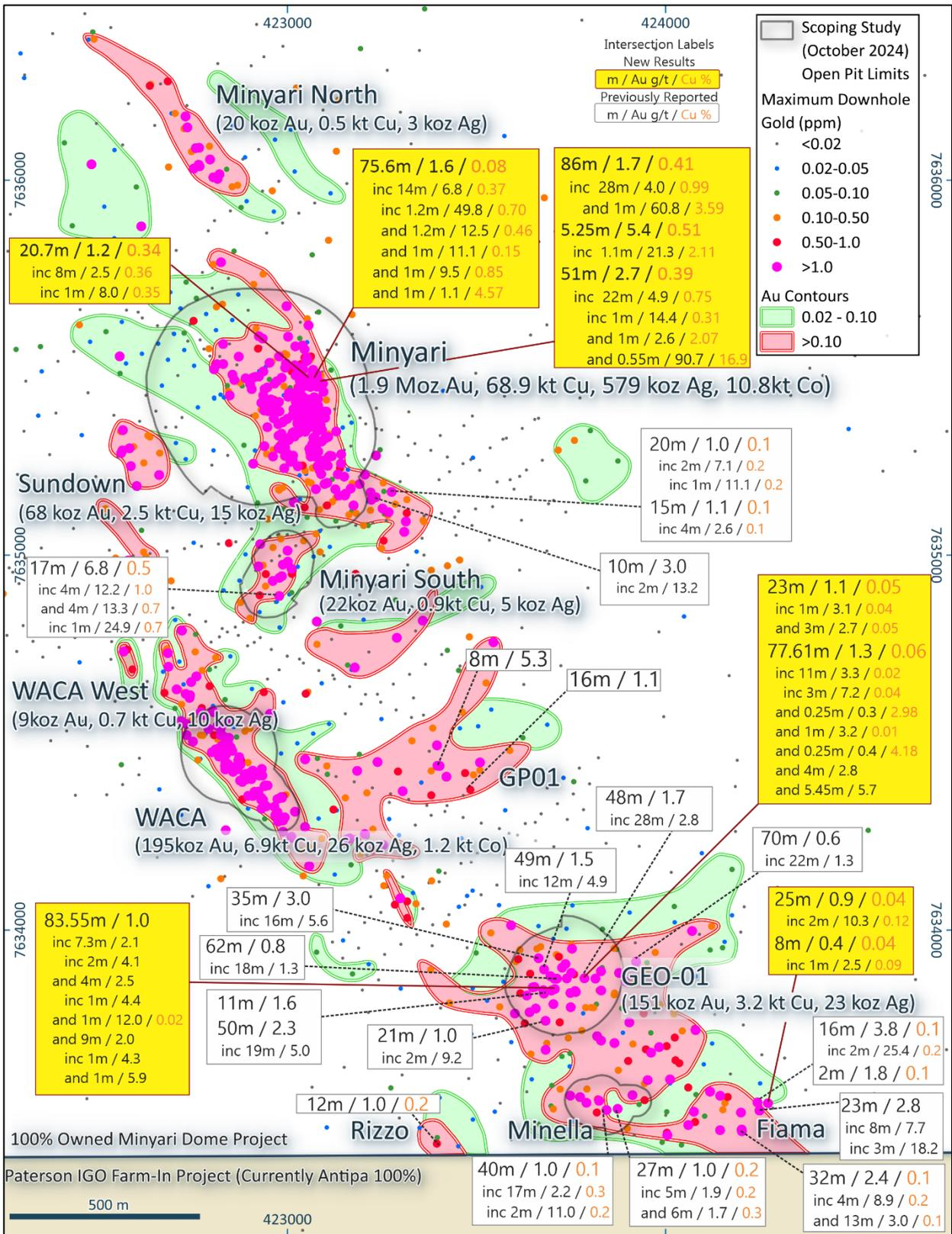
**Figure 2: Map showing the Minyari Dome resource locations, 2024 Scoping Study Update open pit design limits, prospect locations including Minyari South, GEO-01, Fiamo, Minella, and contoured maximum down-hole gold drill results. NB: Regional GDA2020 / MGA Zone 51 co-ordinates, 1km grid.**
