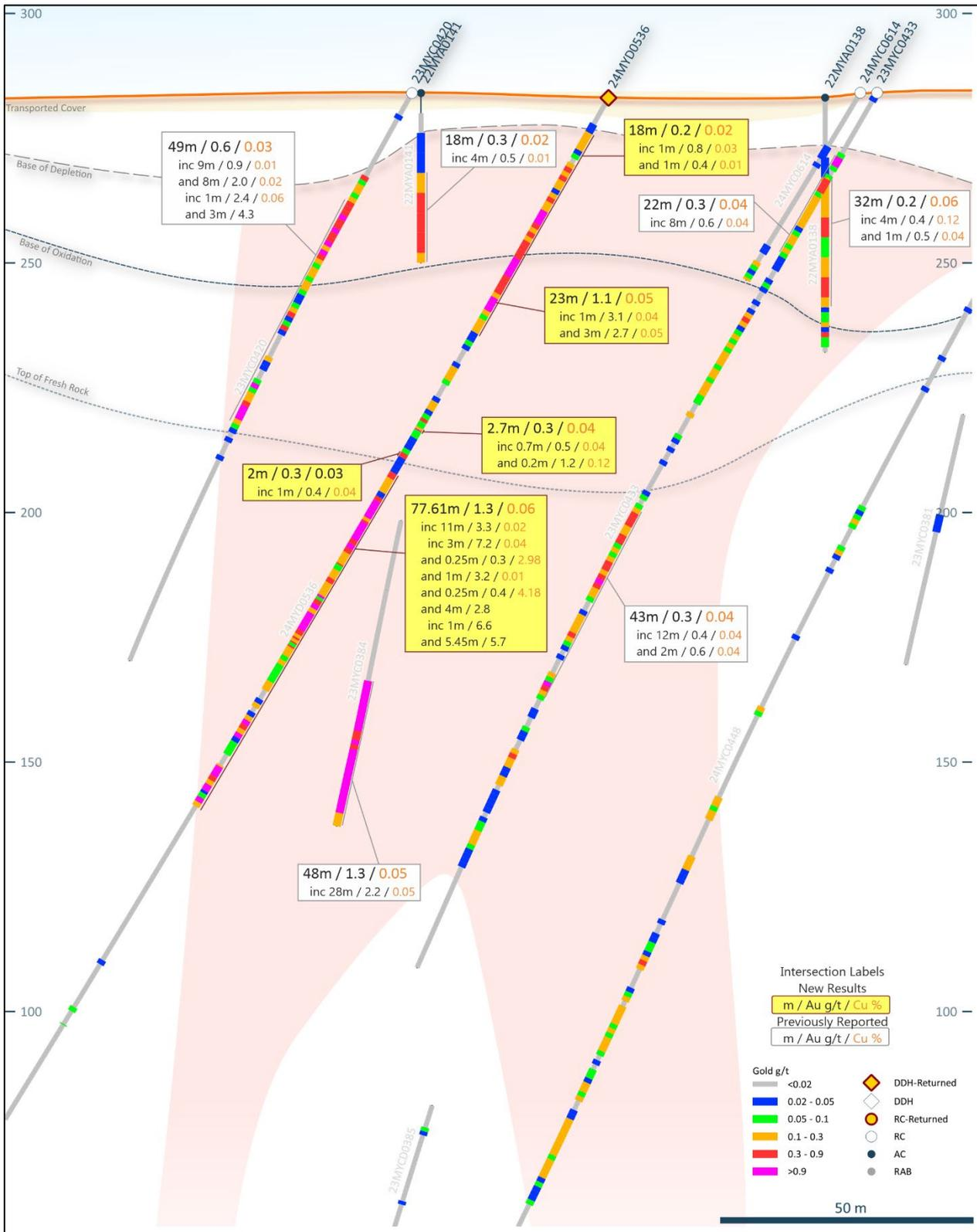
Figure 6: GEO-01 Main Zone deposit drill hole 24MYD0536 NW-SE cross-section (refer to Figures 1, 2 and 5 for location) showing gold±copper drill intercepts, with the deposit open down dip and along strike for multiple zones of mineralisation. NB: 100m elevation (RL), looking toward 035° GDA2020 / MGA Zone 51 Grid.
