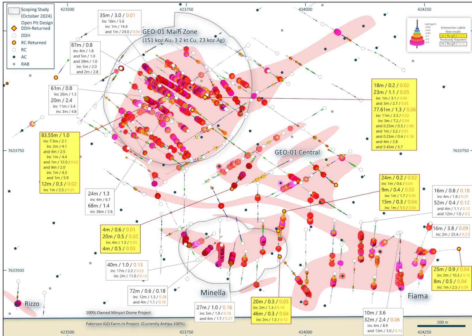
Figure 5: GEO-01, Fiamo, Minella and GEO-01 Central deposits plan view showing gold ± copper drill annotation and intersections and interpreted mineralisation envelopes. Folded and/or faulted hard/brittle quartzite and mafic (dolerite) intrusives are preferentially mineralised. Multiple zones of mineralisation remain open, including high-grade. NB: Regional GDA2020 / MGA Zone 51 co-ordinates and 250m grid.
