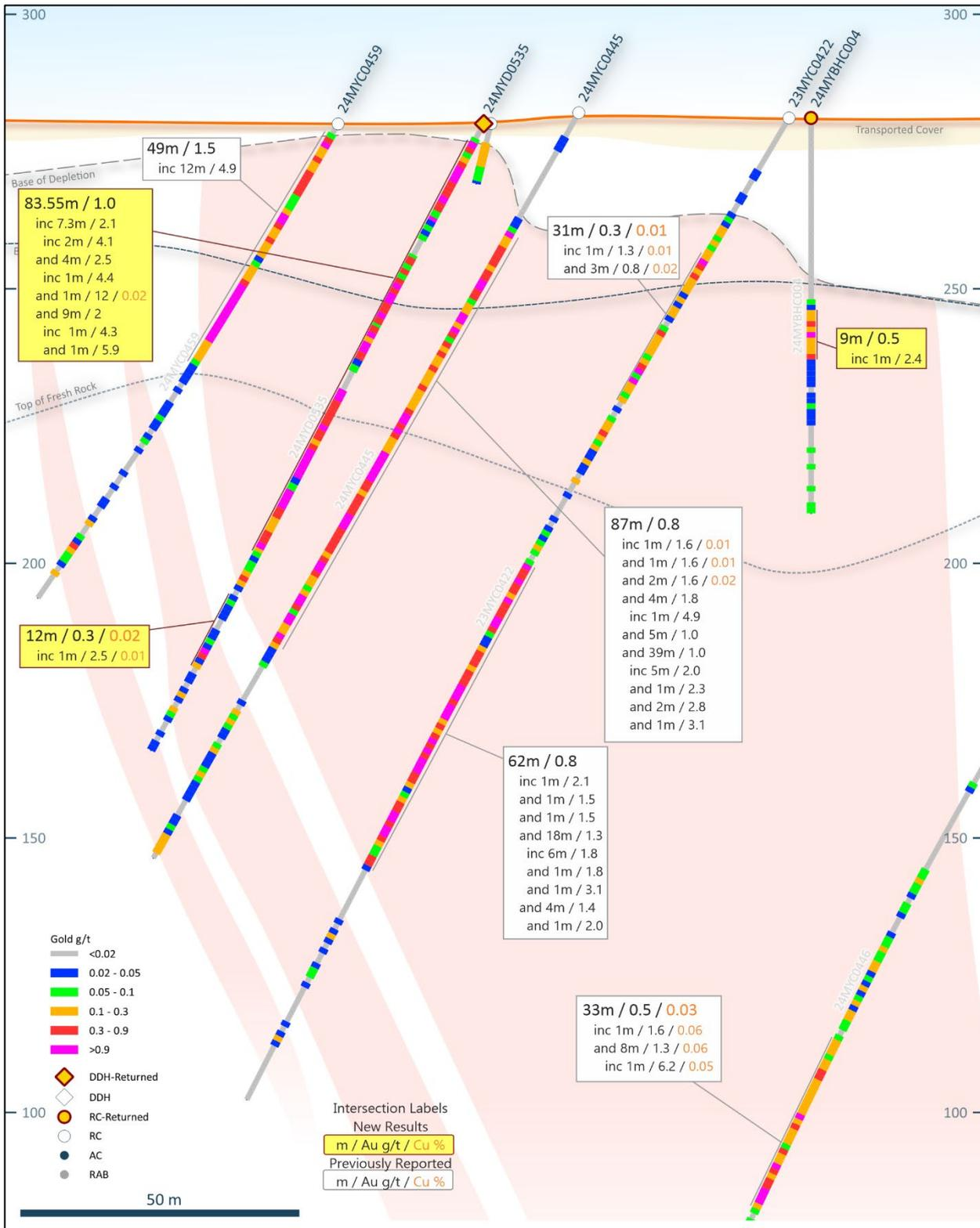
**Figure 7: GEO-01 Main Zone deposit drill hole 24MYD0535 and 24MYBHC004 NW-SE cross-section (refer to Figures 1, 2 and 5 for location) showing gold±copper drill intercepts, with the deposit open down dip and along strike for multiple zones of mineralisation. NB: 100m elevation (RL), looking toward 035° GDA2020 / MGA Zone 51 Grid.**
