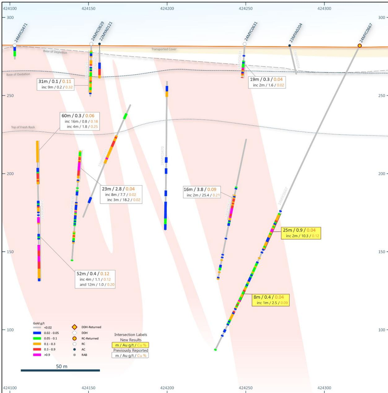
**Figure 8: Fima deposit East-West cross-section 7,633,540mN (refer to Figures 1, 2 and 5 for location) showing gold±copper drill intercepts, with the deposit open down dip and along strike for multiple zones of mineralisation. NB: 50m elevation (RL) and northing grid, looking toward 270° GDA2020 / MGA Zone 51 Grid.**
