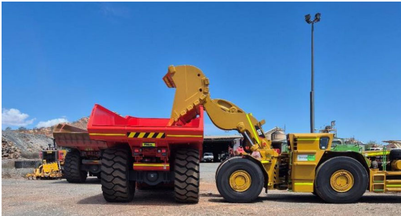
Figure 2: Newly arrived Cat R1700 loader and TH663 dump truck being commissioned on site
