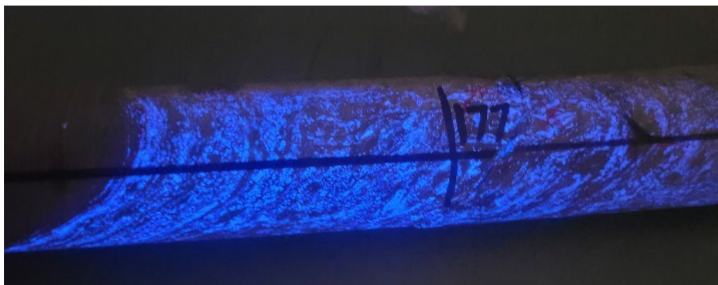
Figure 7 – WQDD013 (0.65m @ 18.35 WO 3 ) scheelite intersection under UV light
