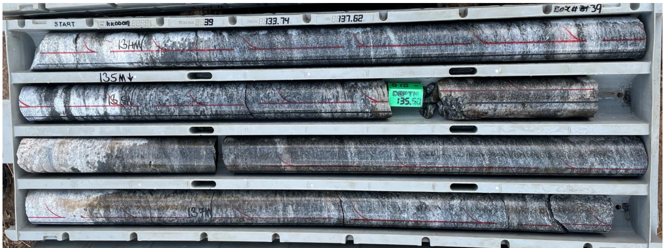
Figure 4. Drill hole KKDD002 showing high-grade disseminated Cu mineralisation (from 133.74m - 137.62m)
