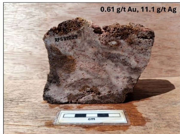
Figure 11: Specimens of silicified limestone (RF531018) and quartz-sulphide veins (RF531029), Singto prospect.
