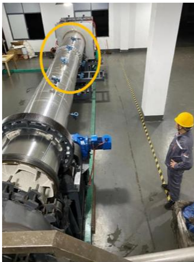
Image 4: Calcining Kiln with temperature gauges highlighted
