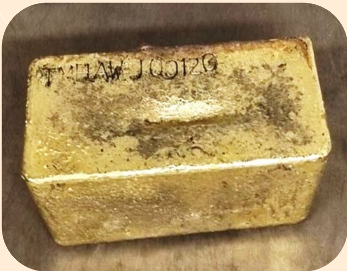
Figure 1. Doré bar at Three Mile Hill Mill
