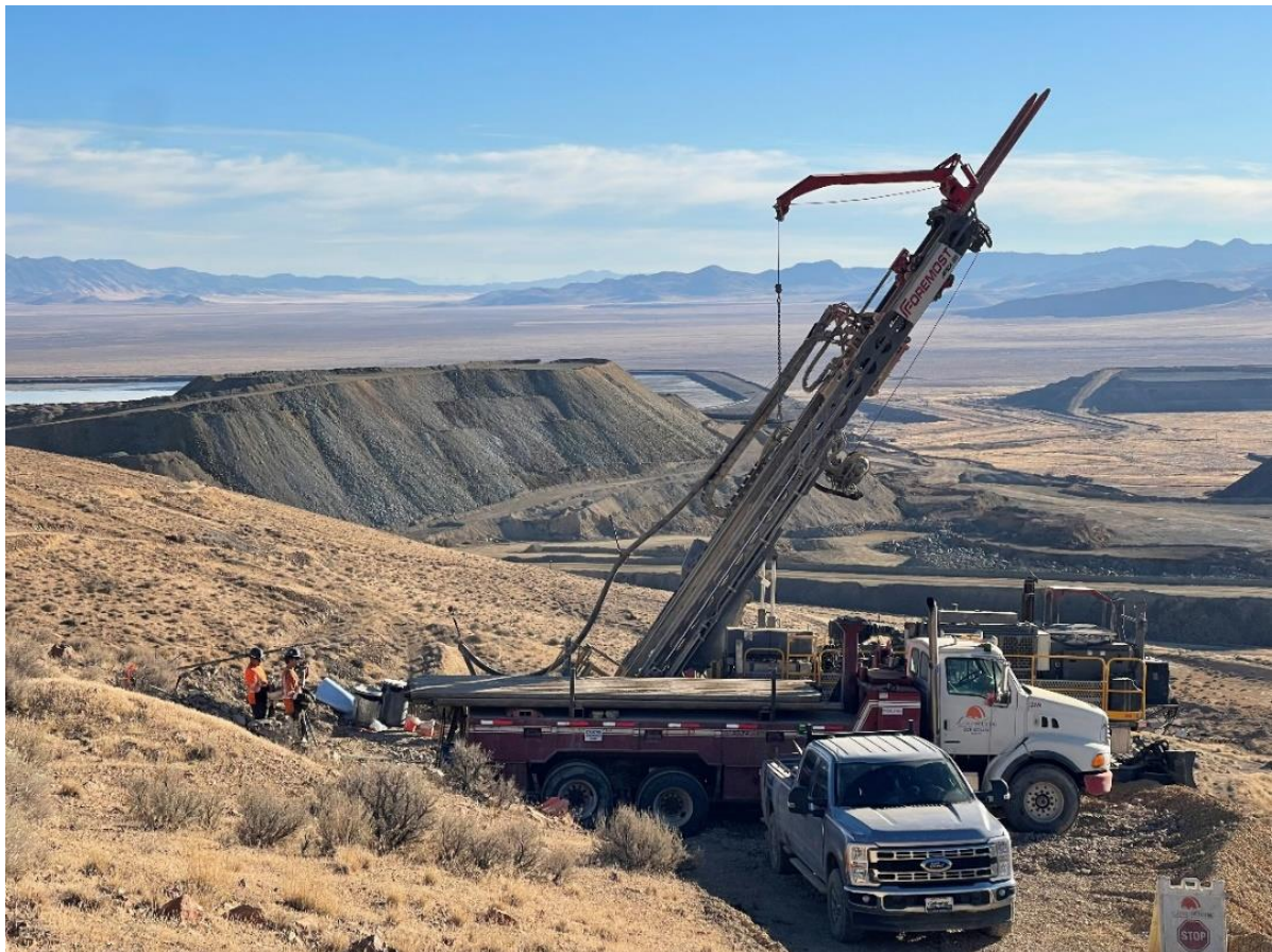
Figure 6: RC drill rig set up ready for drilling at the Independence Project.
