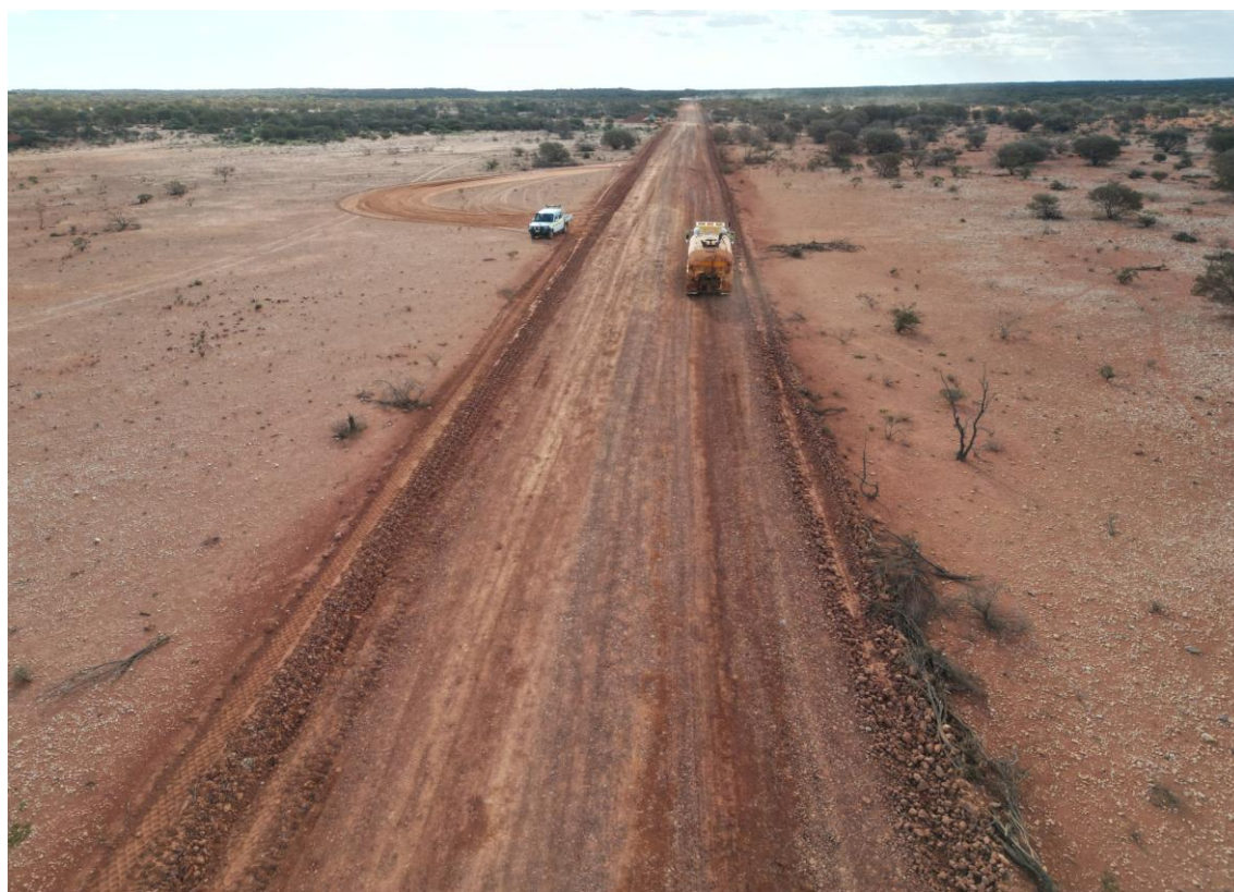
Figure 8: New 20km haul road between the processing plant and the open pit mining area in anticipation of open pit mining fleet mobilising, January 2025.
