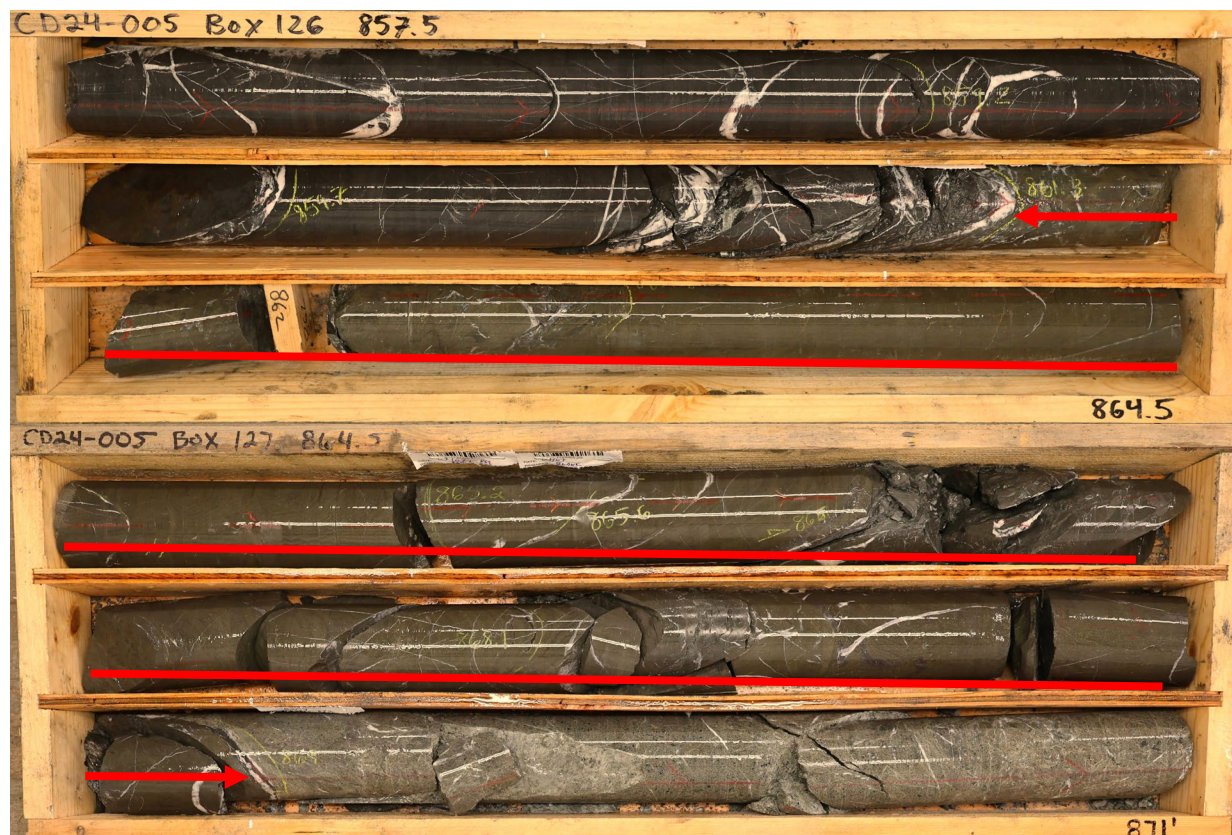
Figure 2. Massive copper sulphide interval in CD24-005 (contains laminated massive sulphides, predominant brassy chalcopyrite thinly interbedded with pyrite and white carbonate veins) from 262.4 to 264.9m assay averaged 6.7% Cu.
