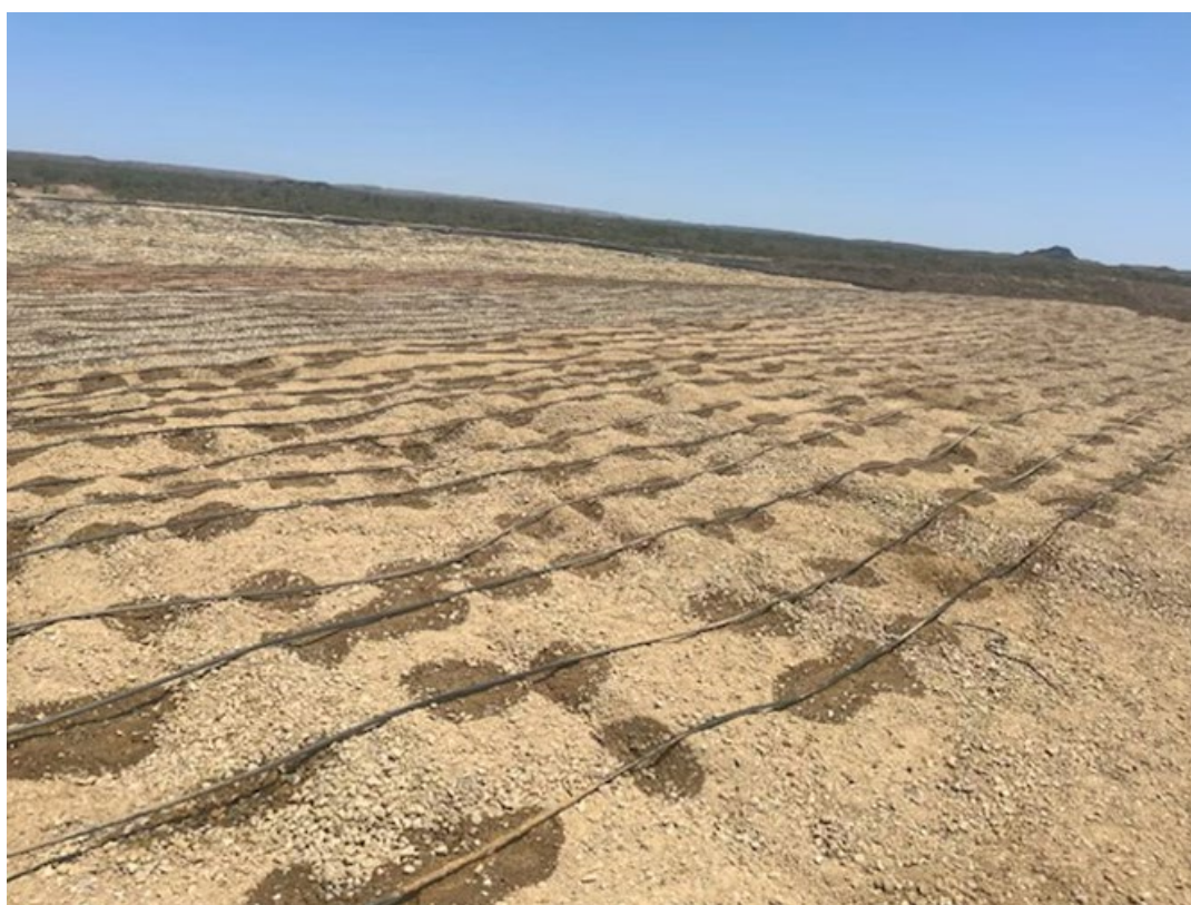
Figure 1. Leach Pad 5 under irrigation on 8 October 2024 at the Cloncurry Operations Hub (COH).
