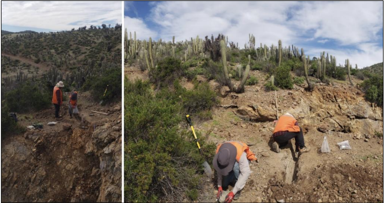
Figure 3: Trenching at an andesite outcrop, mineralisation consists of quartz, iron oxides, and copper oxides. Samples CPO0009117-CPO0009118-CPO0009119 Trench 1 (5.5m at 0.88% CuEq) 2 .
