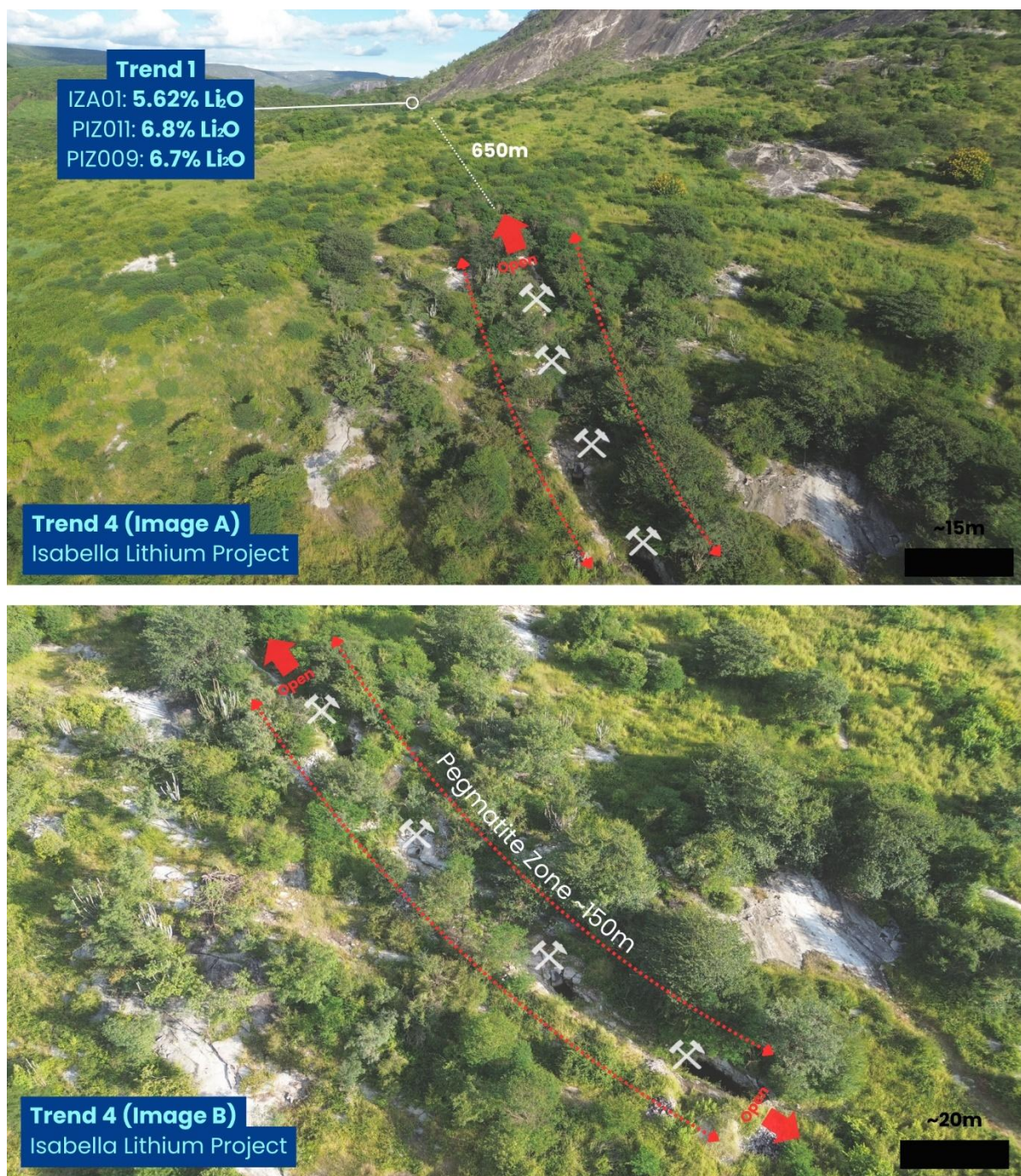
Figure 2: Image A shows the newly discovered Trend 4 in relation to confirmed spodumene mineralisation, while Image B highlights artisanal workings defining the trend at the Isabella Lithium Project.
