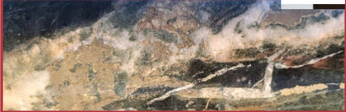
SPD001 221.3m, discrete narrow quartz + magnetite + pyrite vein, 3.6g/t Au (Epithermal)
