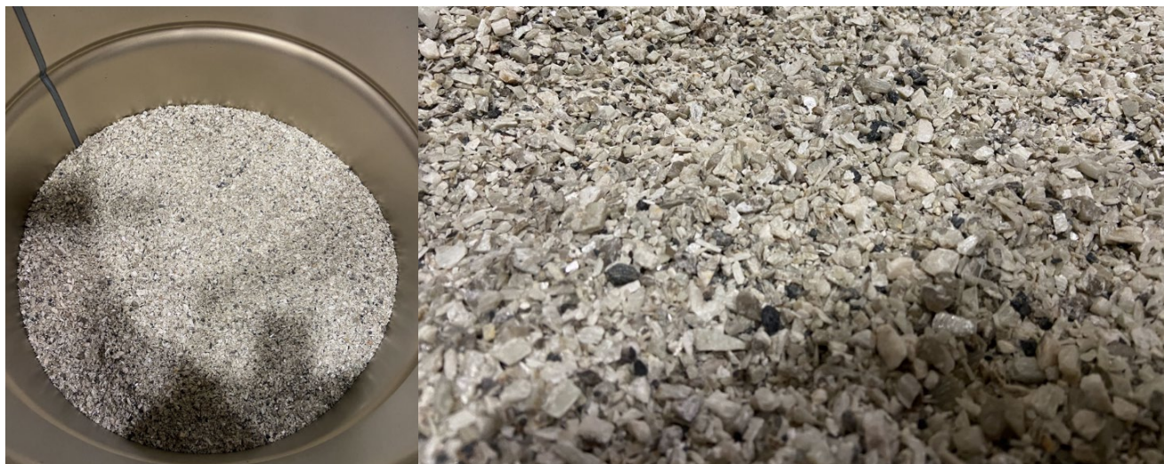
Figure 4: Spodumene Concentrate shipped to EcoPro's Korean Laboratory
