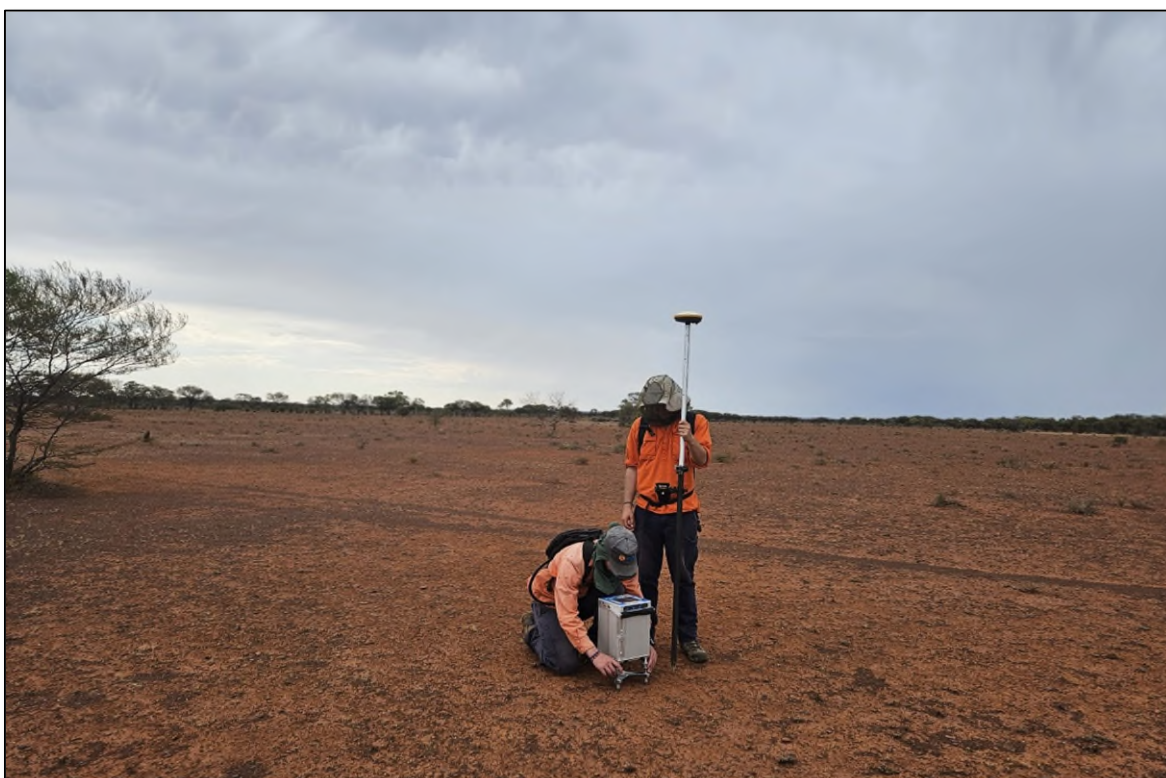
Figure 2: Gravity survey at the Ilgarari Copper Project.
