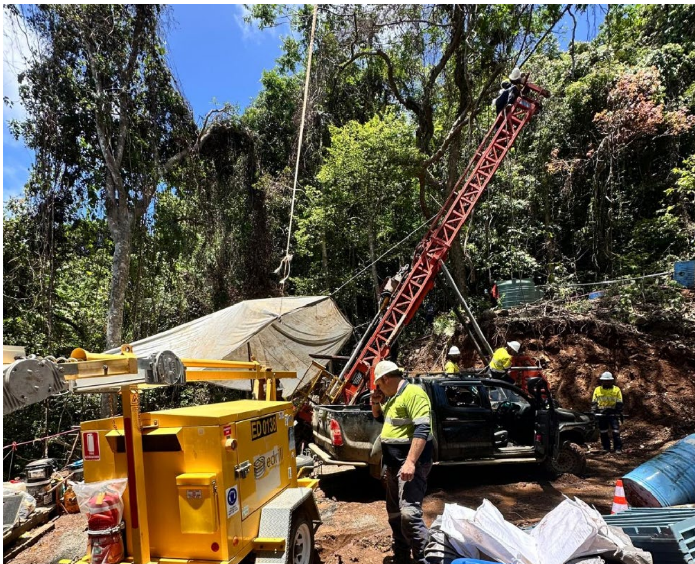
Image 1 – Diamond drilling at Viani
