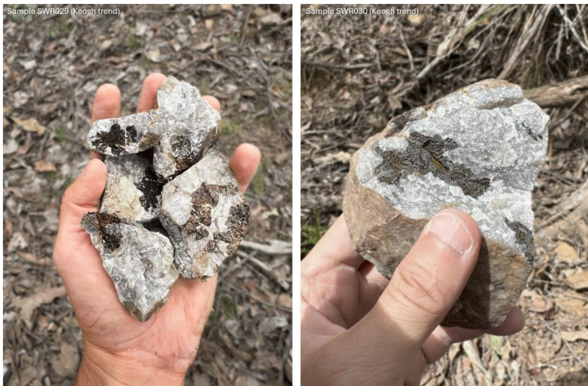
Figure 1. Large cassiterite (tin-oxide) dark mineral crystals and aggregates, from the Sweetwater area: L) Sample SWR029 (16.70% SnO 2 ) and R) Sample SWR030 (8.65% SnO 2 )
