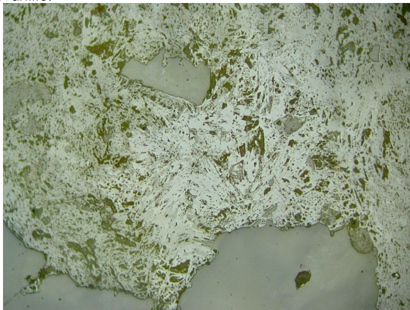
Figure 16: Supergene Sb oxide phases with residual quartz. Plane-polarized reflected light, field of view 2 mm.
