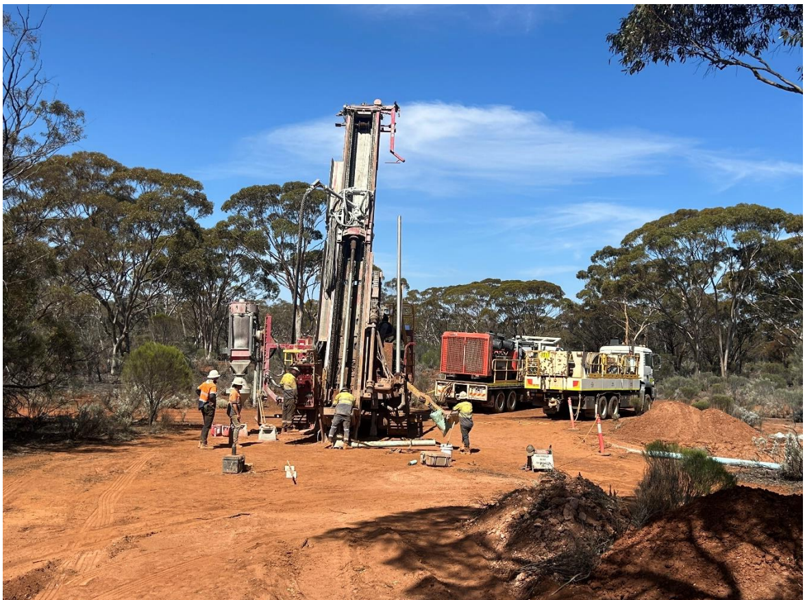
Figure 3: Topdrill RC rig drilling at the Ada Ann Prospect during the previous drilling campaign.
