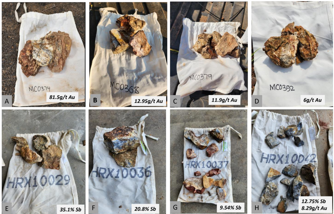
Figure 3: Photo collage for selected samples showing A: MC0374 with 81.5g/t Au, 11g/t Ag, 9840ppm As, 3870ppm Pb, 1275ppm Sb, and 568ppm Zn; B: MC0368 with 12.95g/t Au and 1g/t Ag; C: MC0379 with 11.9g/t Au, 3g/t Ag, and 2890ppm As; D: MC0392 with 6g/t Au, and 3460ppm As; E: HRX10029 with 35.1% Sb, 1.2g/t Au and 4g/t Ag; F: HRX10036 with 20.8% Sb, 0.3g/t Au and 2.2g/t Ag; G: HRX10037 with 9.54% Sb, 1.8g/t Au and 2.5g/t Ag; and HRX10042 with 12.75% Sb, 8.29g/t Au and 1.73g/t Ag. Sample descriptions are provided in Table 1, Appendix 1.
