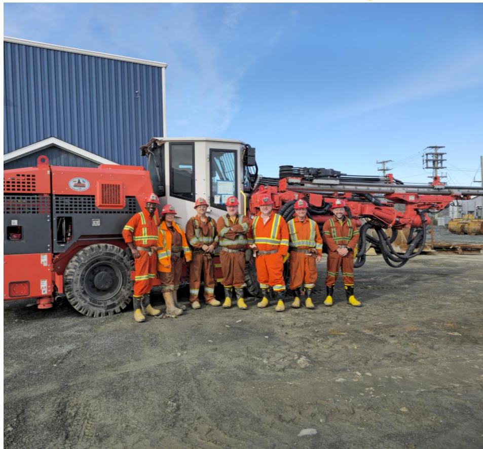
Twin boom jumbo at the Ming Mine
