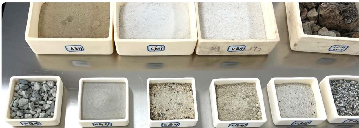
**Figure 13: Various Spodumene Concentrates from around the world showing various particle sizing and grades**
