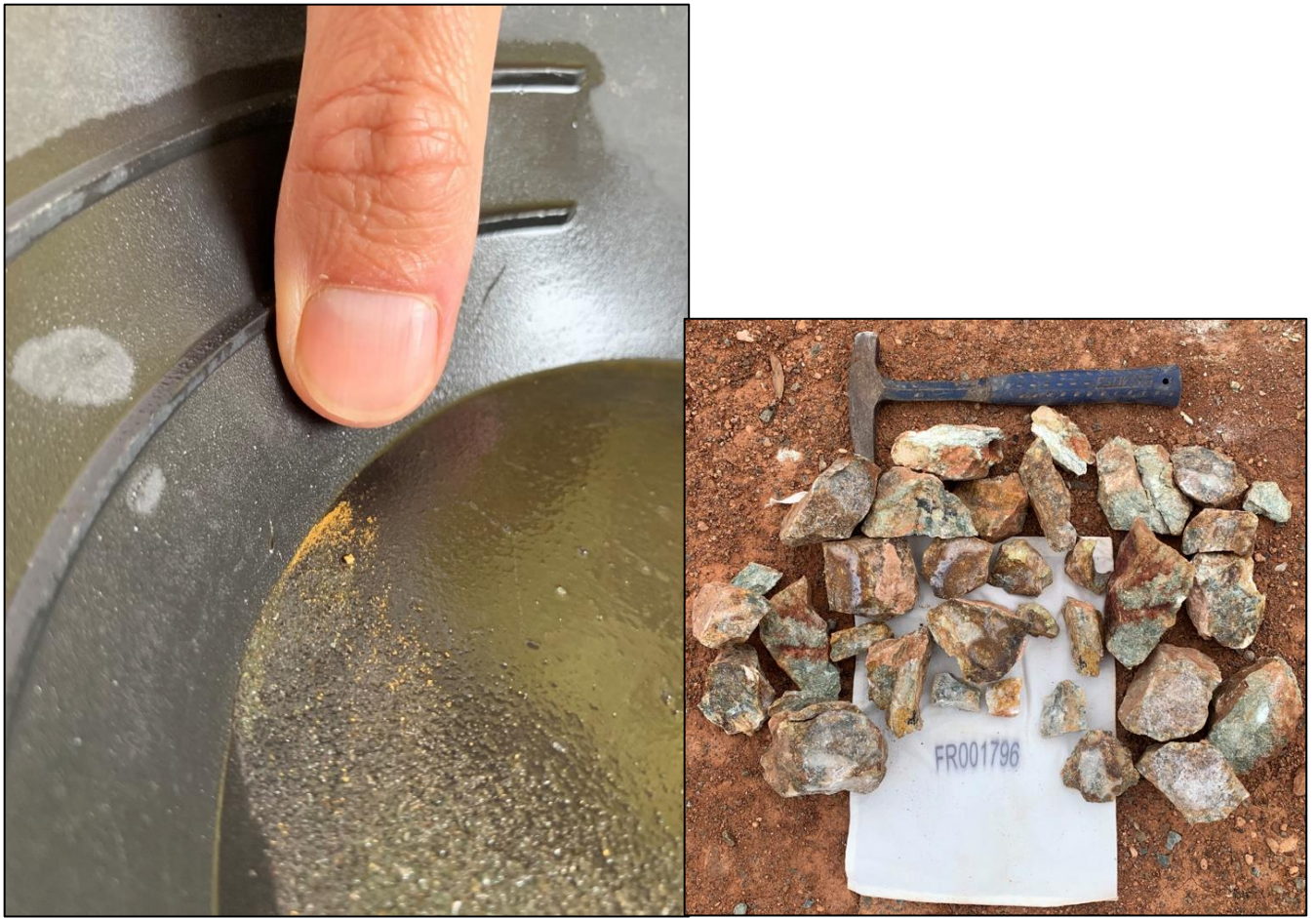
Figure 4. Free gold, panned from rock samples (FR001796) collected at Ada Ann from historic mining waste. Note: visual estimates of mineral abundance should never be considered a proxy or substitute for laboratory analyses where concentrations or grades are the factor of principal economic interest. Visual estimates also potentially provide no information regarding impurities or deleterious physical properties relevant to valuations or the commercial viability of projects.
