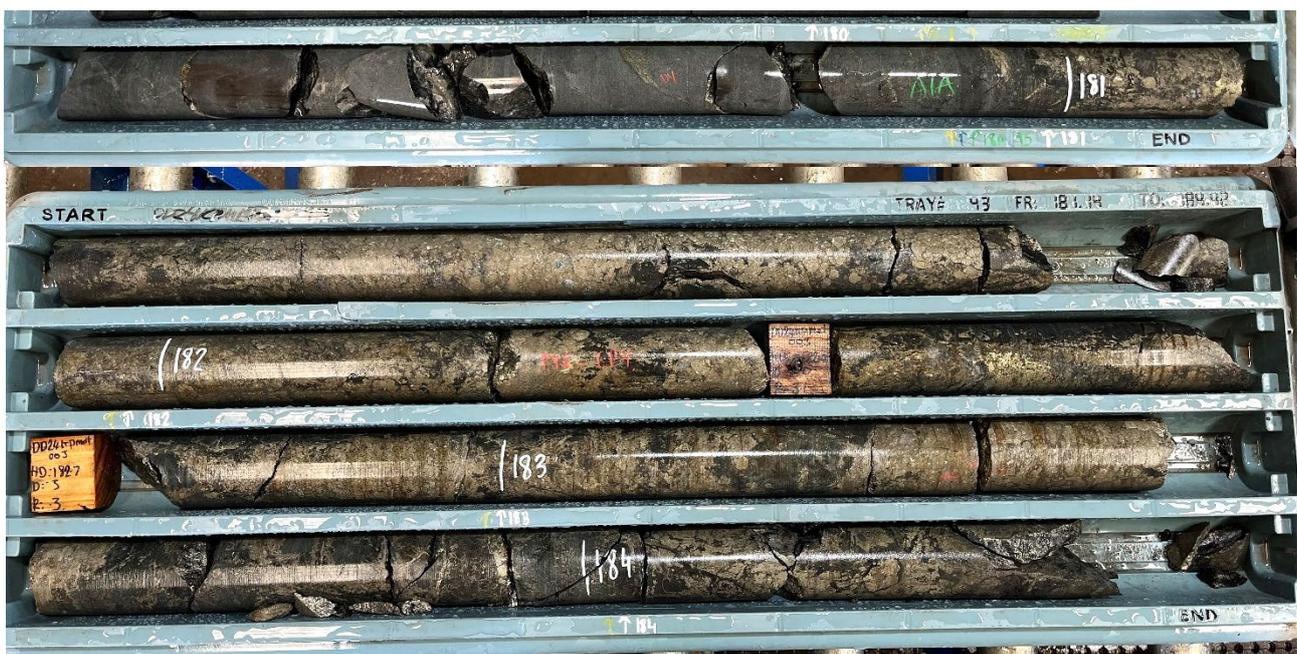
Figure 1: DD24KPMET003 displaying semi massive to massive pyrite-chalcopyrite mineralisation from approximately 181m downhole (assays pending).
