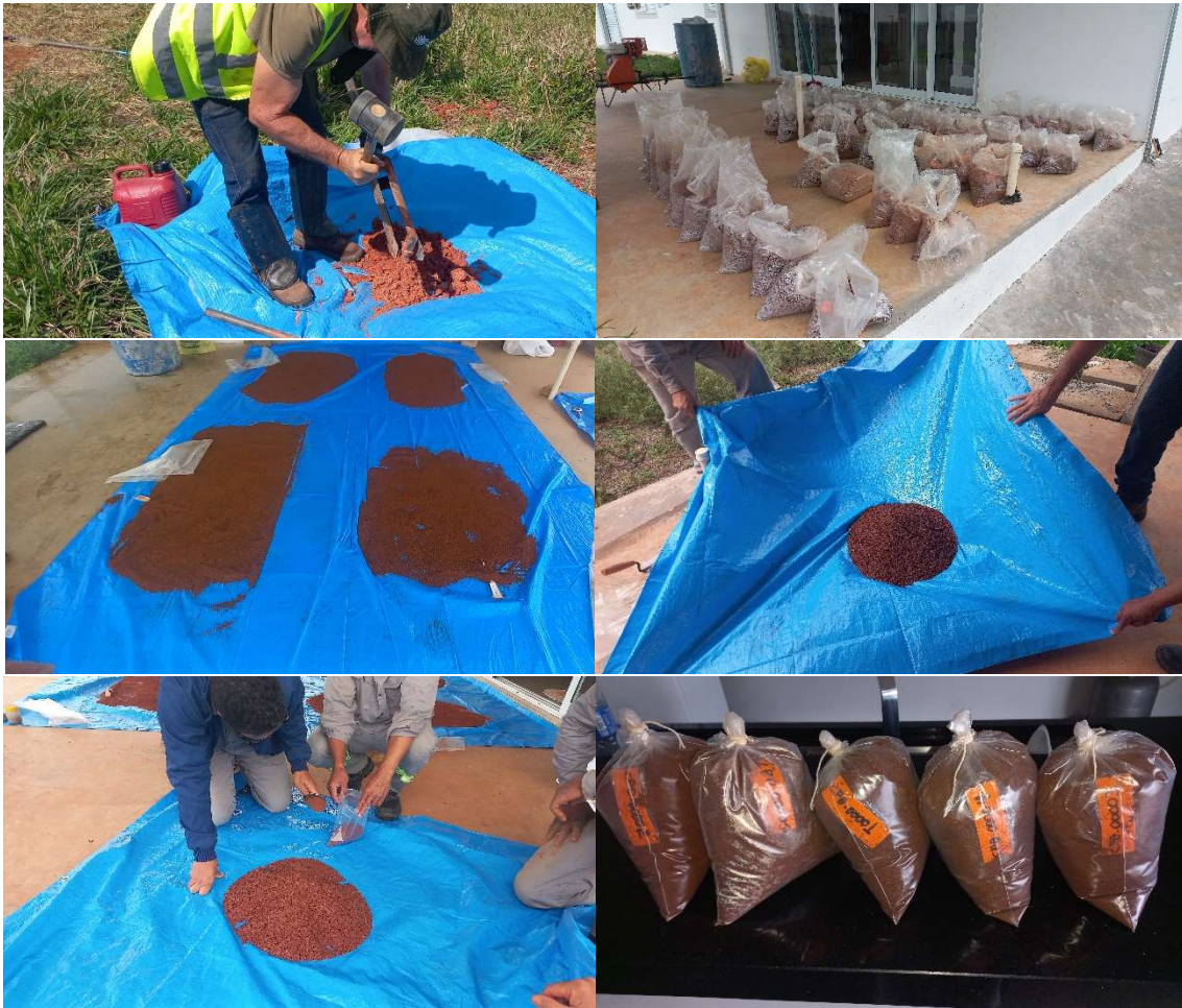
Figure 5: Sequence of images illustrating: (1) Sample retrieval from within the auger's shell, (2) Bags containing material corresponding to 1 meter of depth advancement, (3) Samples exposed to sunlight for moisture reduction, (4) Manual quartering, (5) Separation of an aliquot of approximately 2 kg, (6) Samples ready for dispatch to the SGS laboratory."
