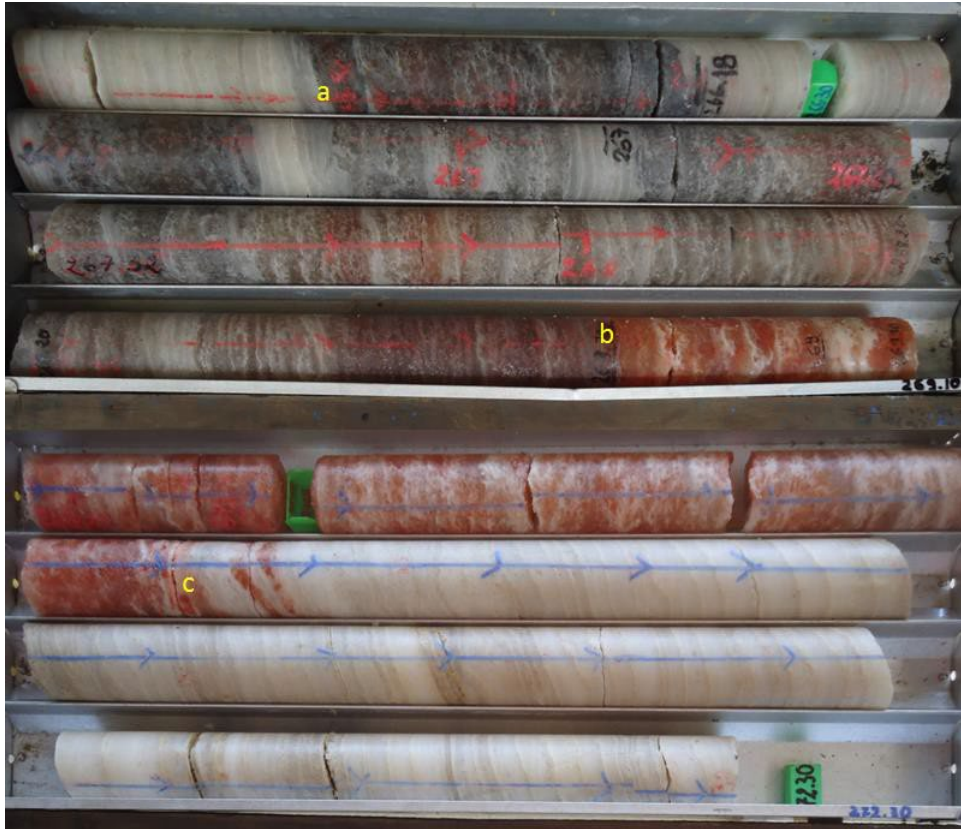
Figure 16. Photograph of (PQ size) core from an intersection of Upper Seam in drill-hole EK_38. The seam is partially replaced; the upper part of the seam (a to b) is Sylvinitite (USS) and the lower part (between b and c) is Carnallitite (USC). Classified as 'type B' seam (as per Table 4 below). The easily identifiable and abrupt nature of the contacts is visible.
