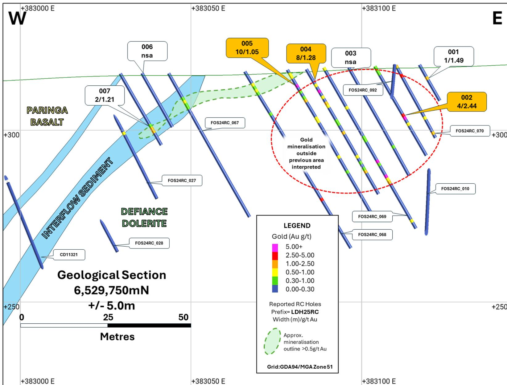
Figure 7: Geological cross section 6,529,750mN
