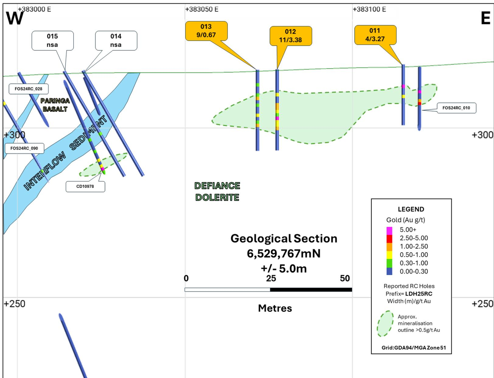
Figure 6: Geological cross section 6,529,767mN
