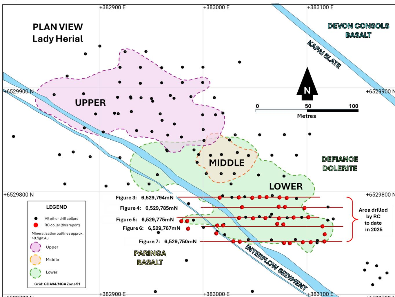
**Figure 1:** Plan view at the Lady Herial deposit scale, illustrating area drilled in latest RC program and location of following **Figures 3** to **7**.
