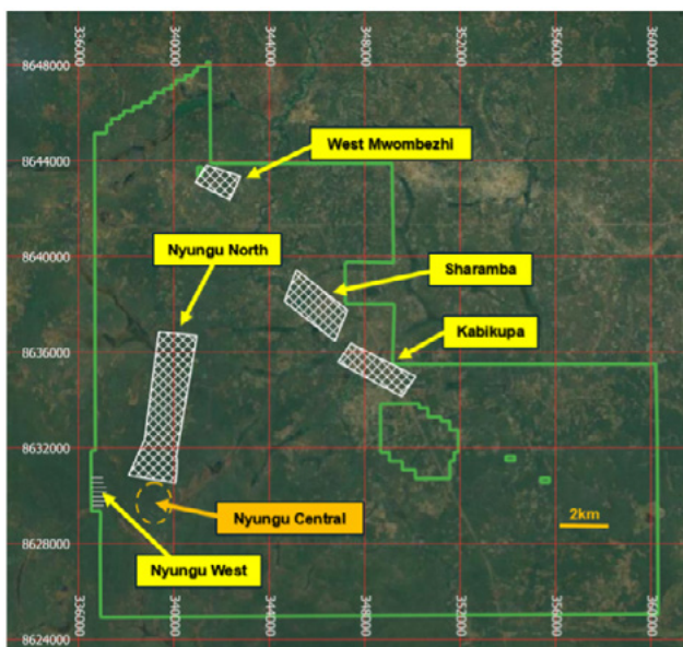
Figure 3. Mumbeshi exploration licence showing grid locations of IP surveys in relation to the Nyungu Central copper deposit (orange ellipse)
