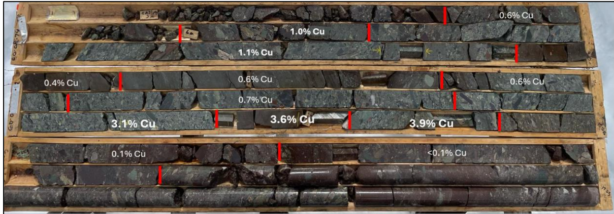
Figure 3. Core photo of GO-08-79 from 3 m to 17.25m showing sampling intervals and assay results (refer Appendix 1). Broken core with core loss occurs from 3 to 5m above the commencement of sampling
