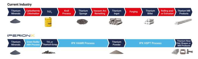
Our HAMR process produces low-cost titanium powder directly from either recycled titanium scrap or domestic mineral feedstock—completely eliminating the need to make titanium metal ingots. Instead, IperionX makes a high purity "ingot" in a powder form that transforms into metal products with traditional powder metallurgy techniques and our HSPT<sup>TM</sup> process.
