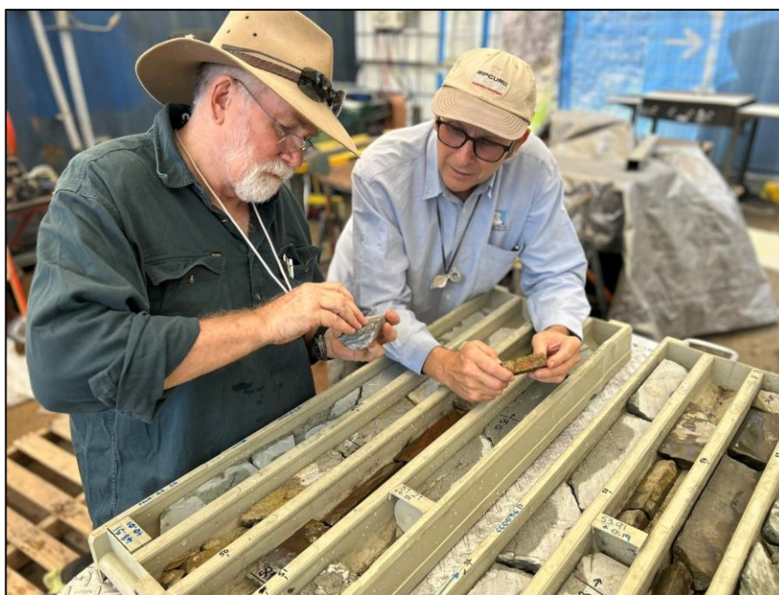
Figure 2: Infinity Mining Geologists Dr Matthew White and Dr Darryn Hedger inspecting the pyrrhotite-bearing drill core samples associated with copper mineralisation in hole CC0036D.
