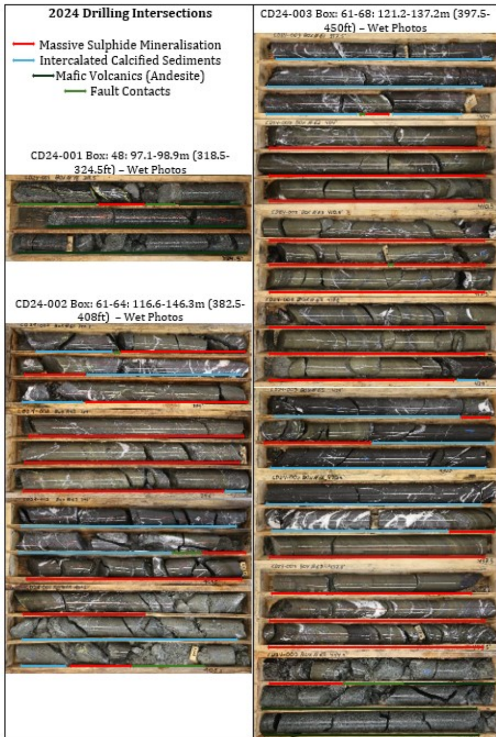
Figure 6. Massive sulphide mineralised intercepts in all core boxes from holes CD24-001, CD24-002 and CD24-003
