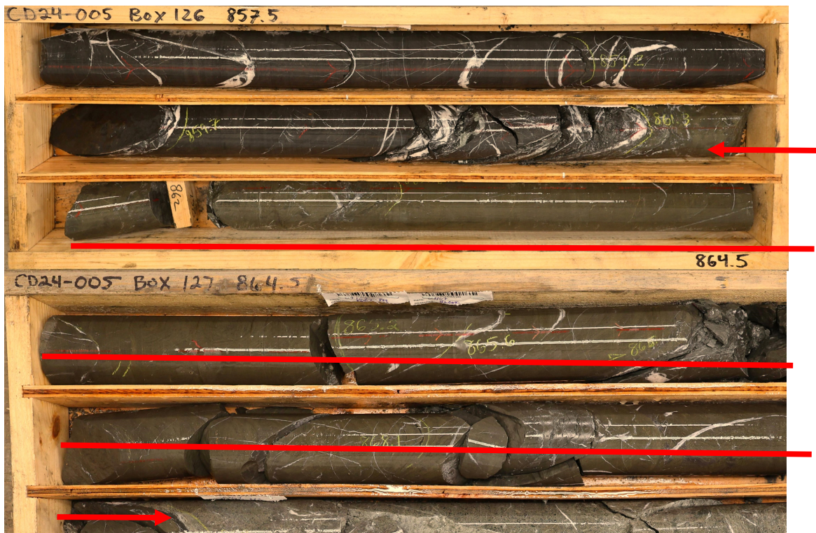
Figure 5. Massive copper sulphide interval in CD24-005 (contains laminated massive sulphides, predominant brassy chalcopyrite thinly interbedded with pyrite and white carbonate veins) from 262.4 to 264.9m assay averaged 6.7% Cu.
