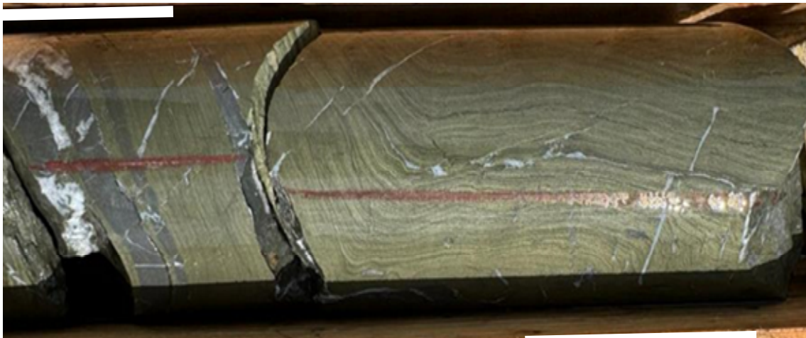
Figure 4. Finely laminated massive iron and copper sulphides at 126.0m depth in drill hole CD24-003. From an 8.1m down-hole intersection which assayed 11.4% Cu and 20.7g/t Ag. Scale bar = 5cm.
