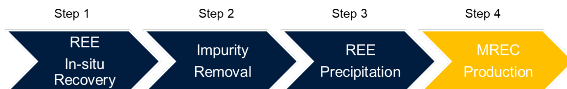
Figure 13. Simple 4 step process flow sheet for ionic clay MREC production at Ema Project
