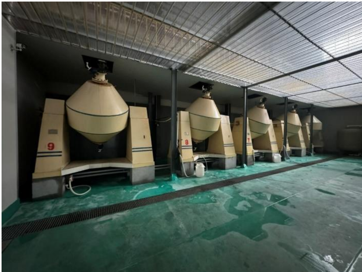
Figure 4: Acid leach in newly commissioned HPQ factory visited in Lianyungang
