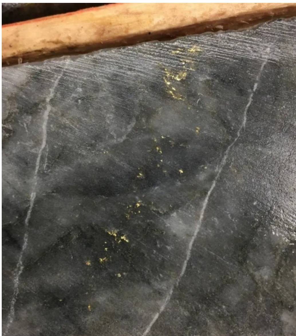
Figure 3: Photo of core from drillhole BO-21-08 at the Paquin East prospect showing Visible Gold within characteristic blue-grey quartz (184.5m). The one metre interval 184-185m assayed 1m@ 129.25g/t Au. This was within 9m @ 16.96g/t Au from 178.5m vii .
