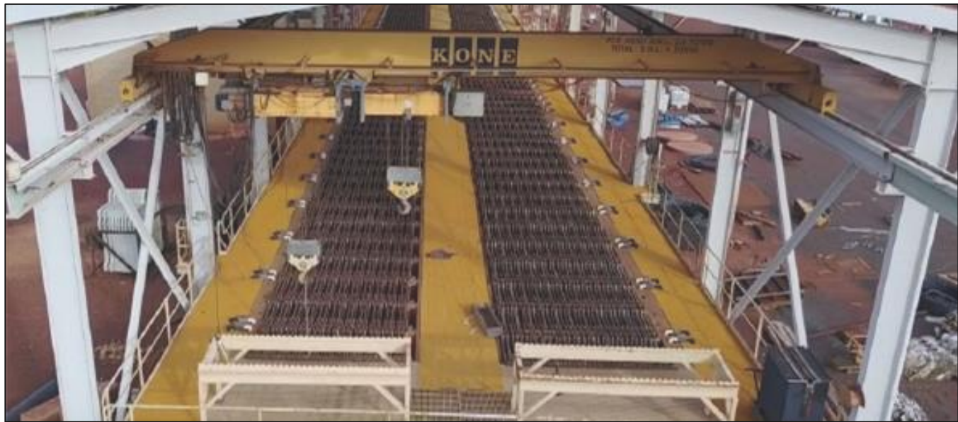
Partial refurbishment of Electrowinning Circuit to operate at 6,000 tpa, well below peak production of 25,000 tpa
