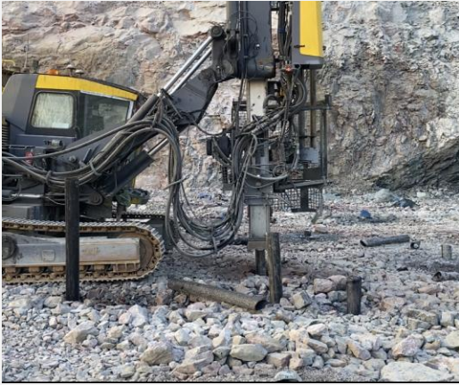
TRADITIONAL PIPING PROCESS WITH POOR BLAST OUTCOMES
