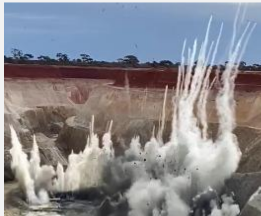
TRADITIONAL PIPING PROCESS WITH POOR BLAST OUTCOMES
