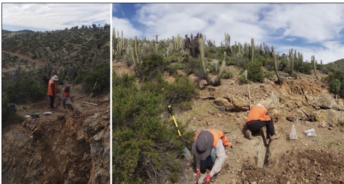
Figure 11: Trenching at an andesite outcrop with silica-albite-sericite alteration within a silicified and brecciated structure. Mineralisation shown to consist of quartz, iron oxides, and copper oxides.
