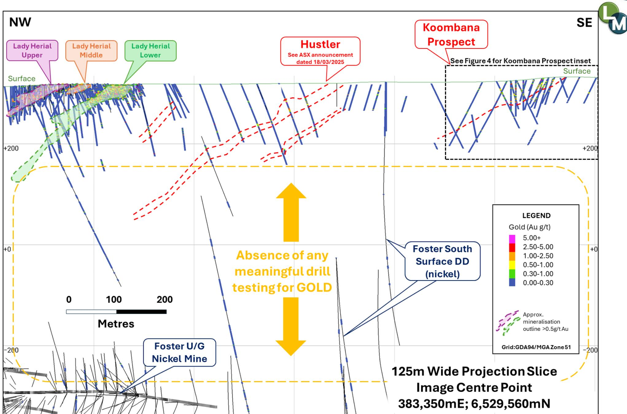
**Figure 3:** Long projection (looking northeast, 125m wide slice) illustrating the relative position of Koombana to Lady Herial, Hustler and the Foster Underground nickel mine.
