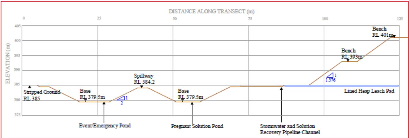
**Figure 6: Extended Heap Leach Plan Cross Section with Ponds, Bunds and Pipeline**
