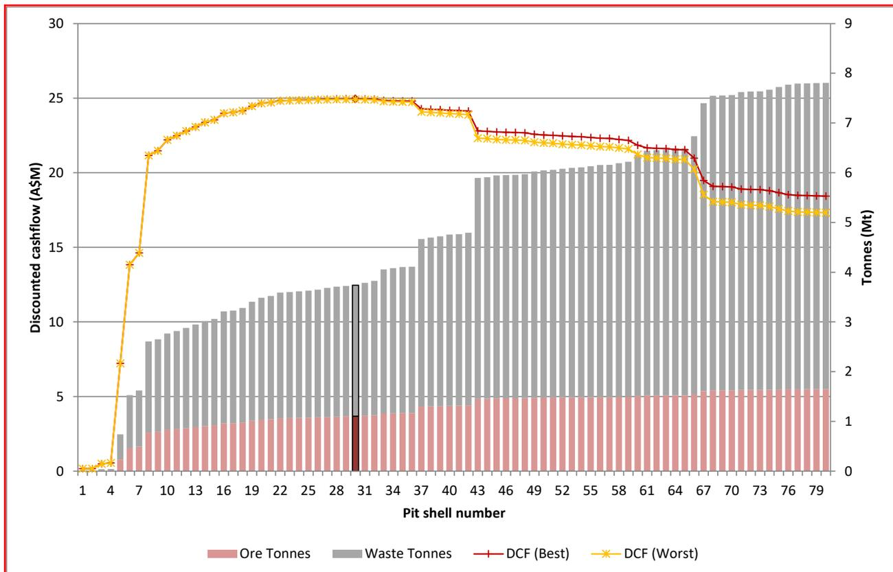
Figure 8: Crawford Oxidised Material Base Case Pit by Pit Graph
