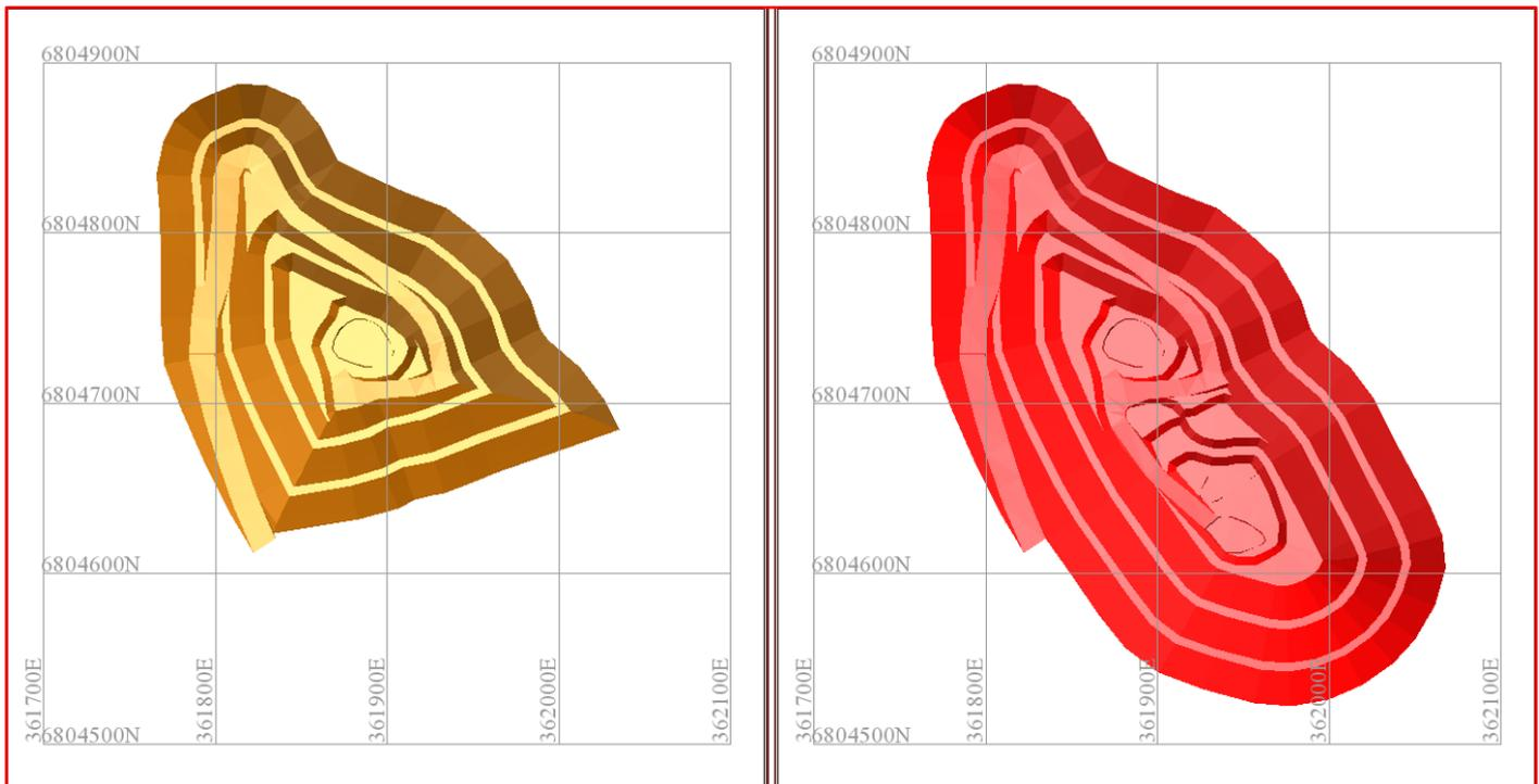
**Figure 10: Crawford Oxidised Material Pit Design Stages 1A (left ) and 1B (right), Plan View**
