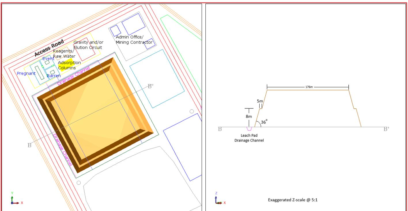
**Figure 5: Heap Leach Plan and Cross Section**
