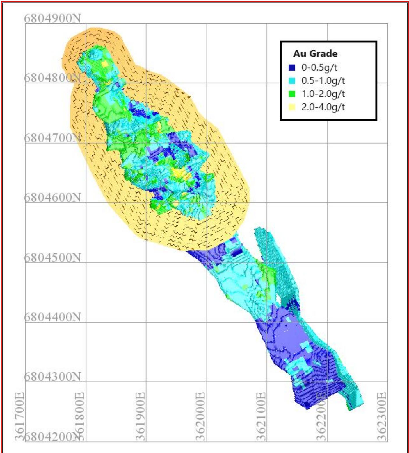
Figure 9: Selected Crawford Oxidised Material Whittle Optimisation Shell (with Domained Resources)
