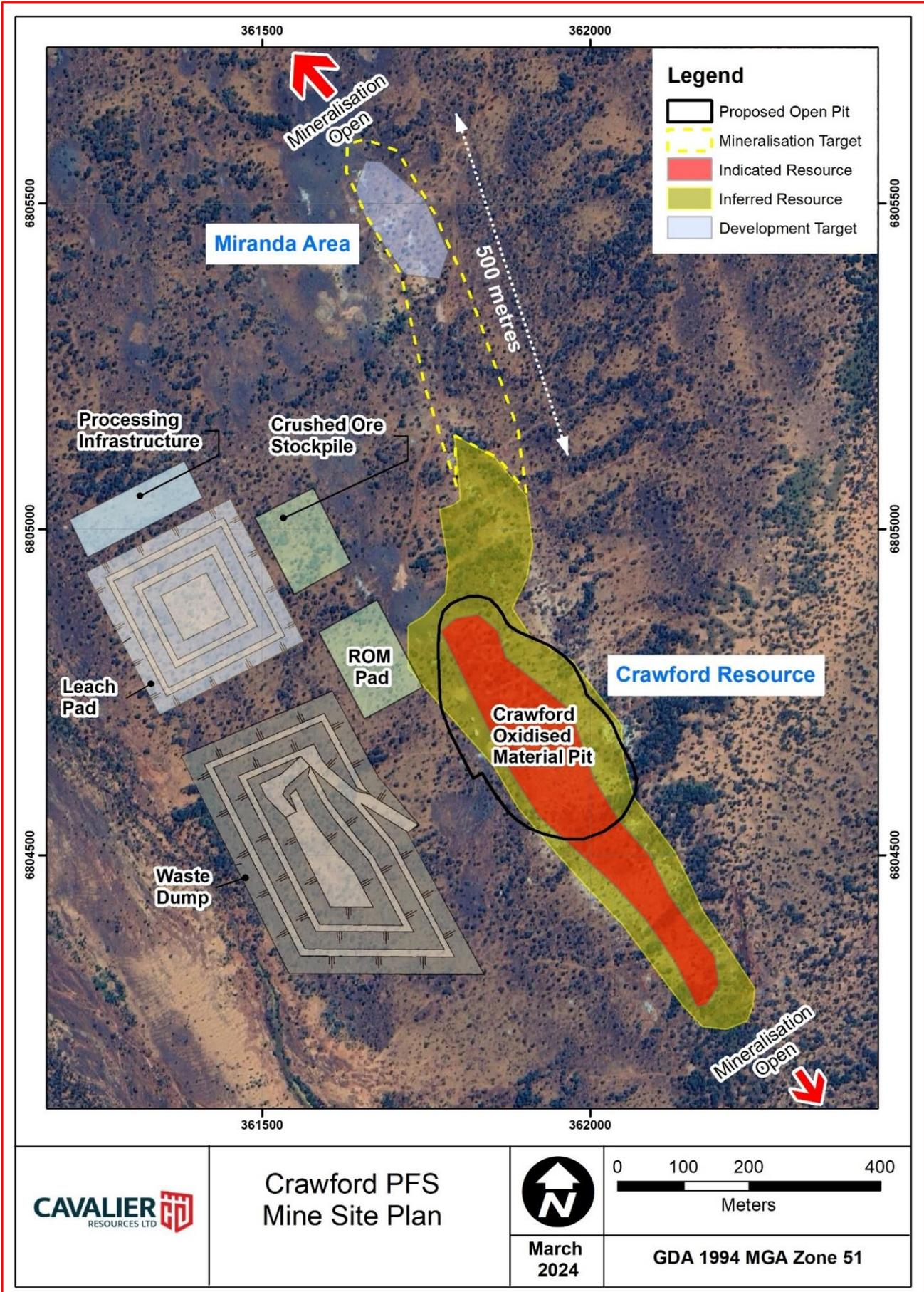
Figure 1: Crawford Gold Project, Stage 1 Simplified Open Pit Site Plan Outlining the Current Resource and Potential Extensions to the Resource and Mining
