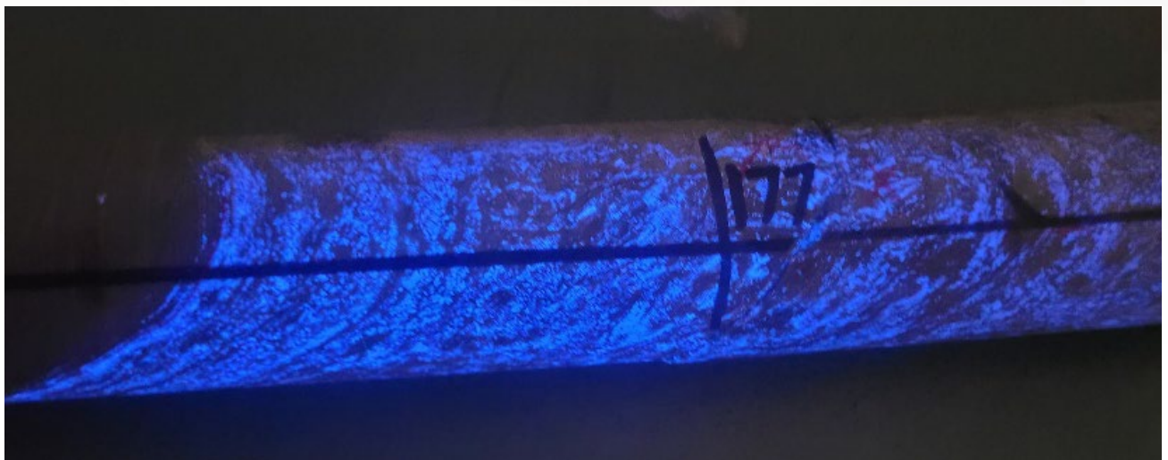
Figure 2 - WQDD013 (0.65m @ 18.35 WO 3 ) scheelite intersection under UV light
