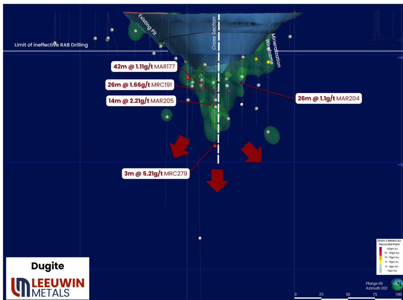
Figure 9 View South of Dugite showing re-modelling of existing drill holes. Drilling is very limited to beneath the existing pit with strike extents not tested, this remains an area for follow up drilling.
