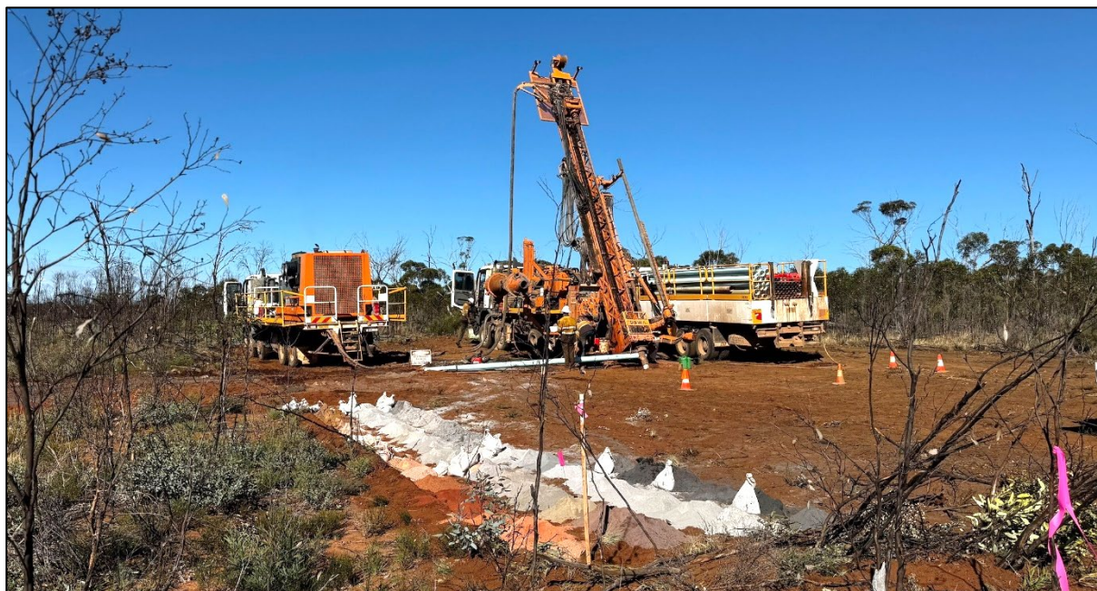
Figure 1: Balladonia Project: Reverse Circulation drilling underway on the first drill-hole
