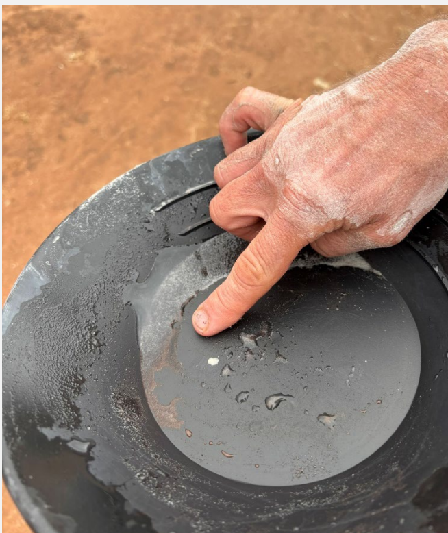
Figure 2. (Left) Panning of cassiterite (grains of dark grey to black material).
