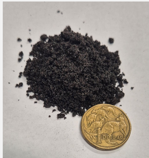
Figure 2. (Left) Panning of cassiterite (grains of dark grey to black material).
