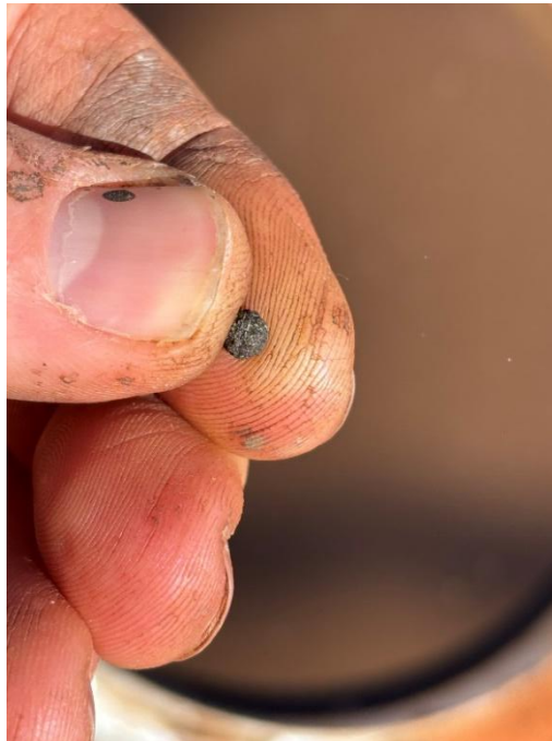
Figure 4: Typical example sulfide nodules from sieved sample at Hatlifter
