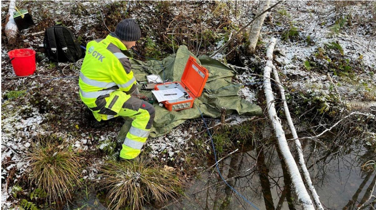
**Figure 2: Installation of magnetotelluric measuring equipment**
