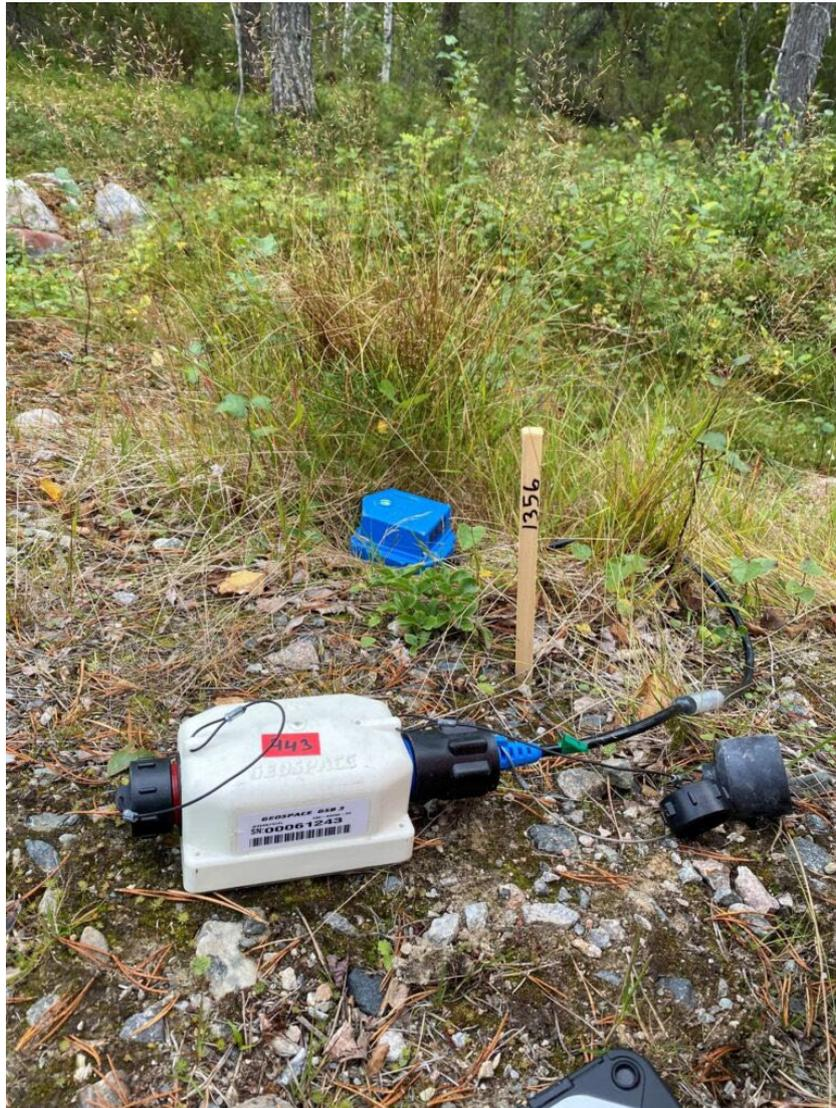
*Figure 3: A geophone for seismic measurement of a dense network installed in the terrain.*
