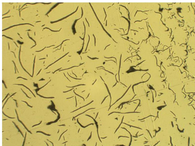
Figure 1 - Photo micrographs of grey cast-iron made with Sarytogan "Micro 80C" Graphite
