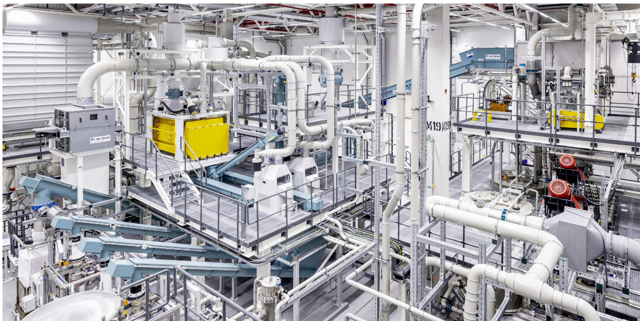
Figure 1 – Part of the Shredding and Beneficiation circuit installed by Primobius at Kuppenheim
